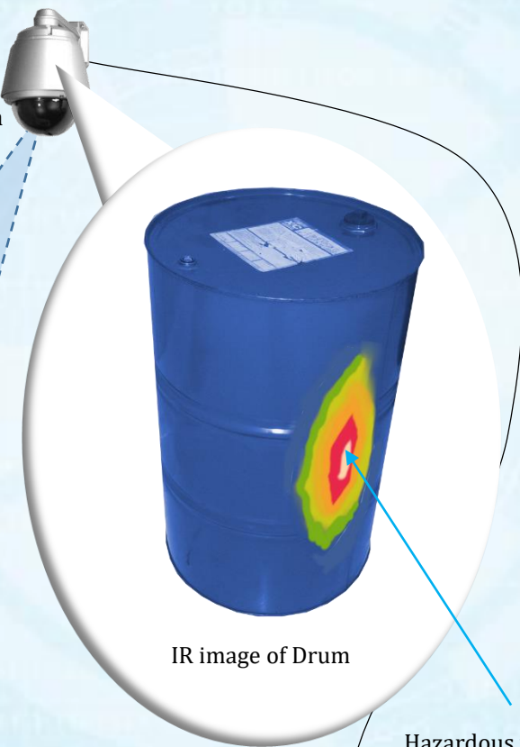
Hazardous material has eaten away at drum creating a leak
