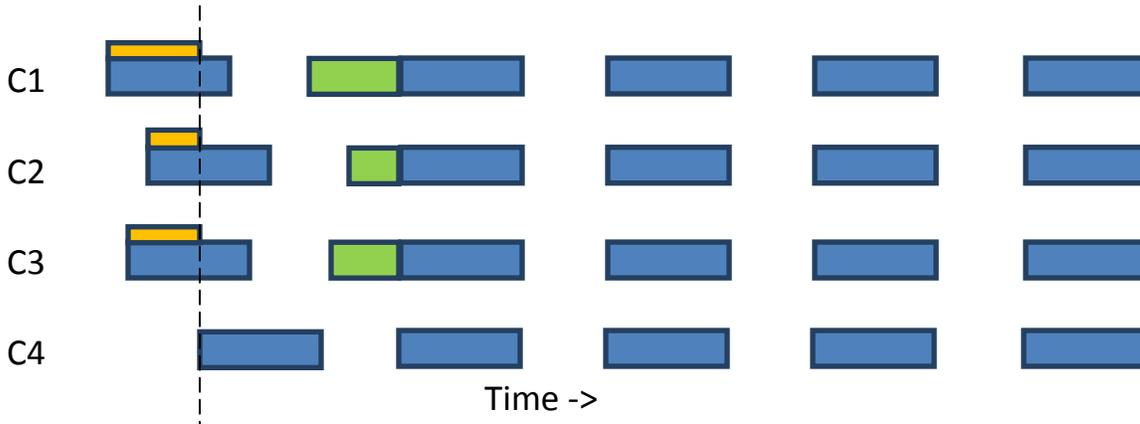
As illustrated above, the blue blocks indicate exposures by the cameras C1-C4. The orange blocks indicate the time that the given camera's exposure is offset from the slowest camera which in this case is camera C4. The synchronization process is about determining these offsets in orange and writing the applicable correction offsets to the "early" cameras to delay the start of the next frame by these correction offsets shown in green above.
