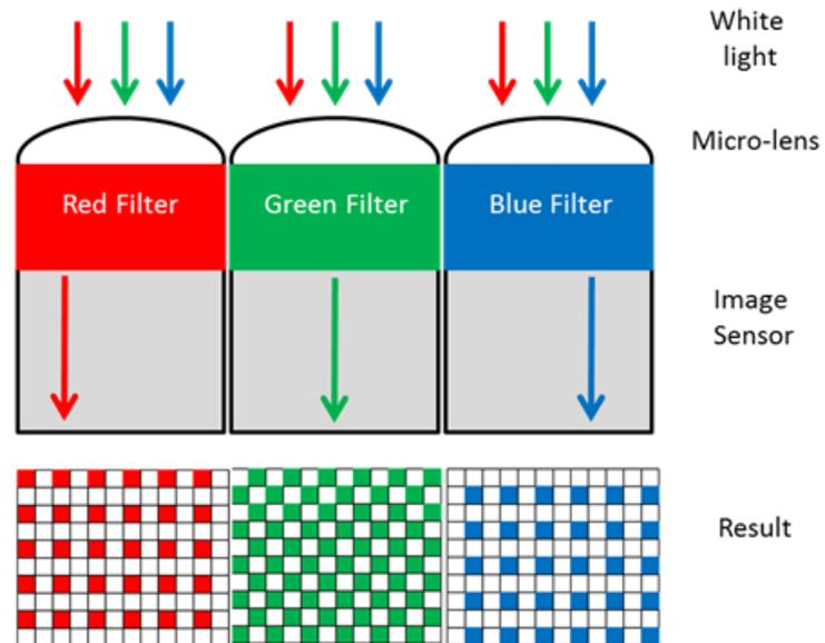
Fig. 2 - Filtering of light on a Bayer sensor
