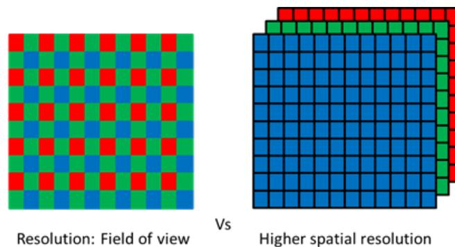
*Fig. 9 - Bayer RGB vs multi-sensor camera resolution*
