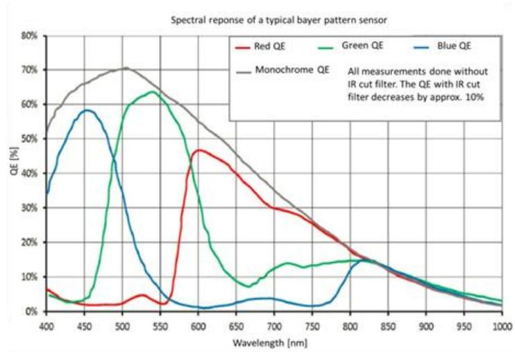
**Fig. 5 - Spectral separation of a Bayer pattern RGB sensor**
