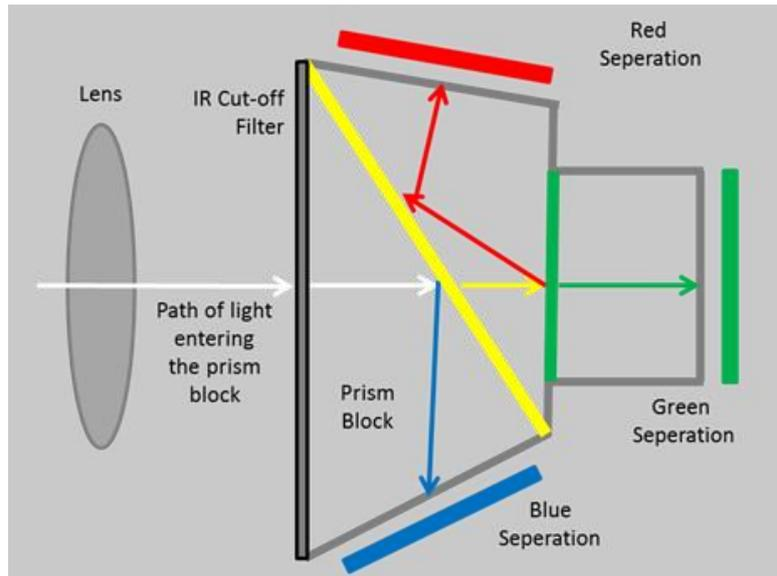
*Fig. 1 - Separation of light inside the prism block*
